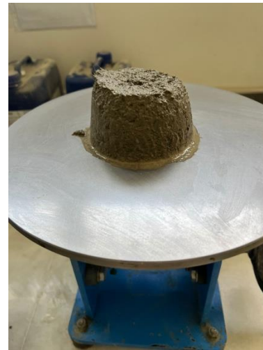
Şekil 2. 6 mm long mortar mixture containing 1% hemp fiber
