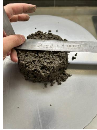
Şekil 1. 12 mm long mortar mixture containing 1% hemp fiber
