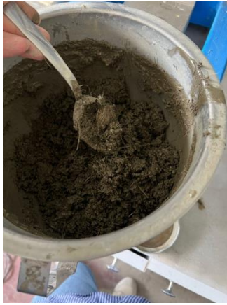
Şekil 1. 12 mm long mortar mixture containing 1% hemp fiber
