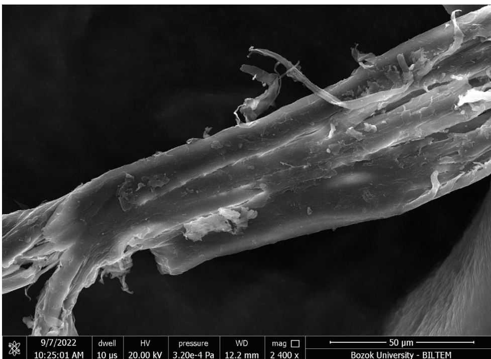
Figure 4. SEM image of the pretreated fiber.
