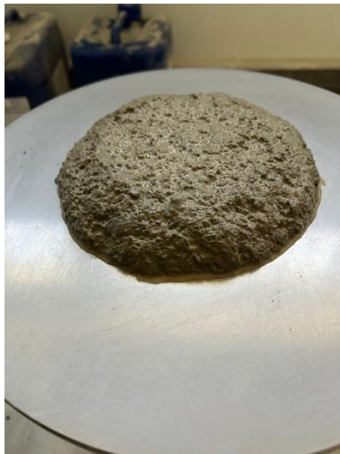
Şekil 2. 6 mm long mortar mixture containing 1% hemp fiber
