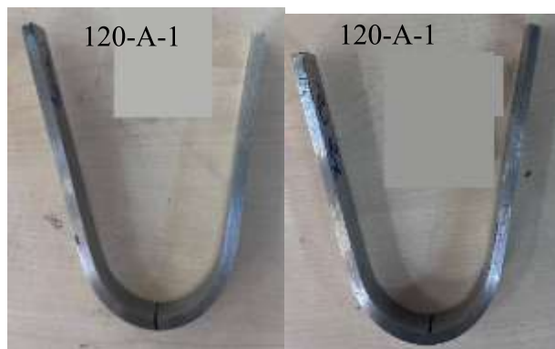
Figure 9 Deformation examination of the samples as a result of three-point bending test.
