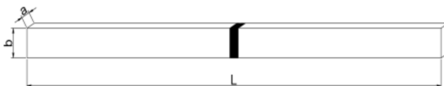
Figure 5 Three point bending test specimen
